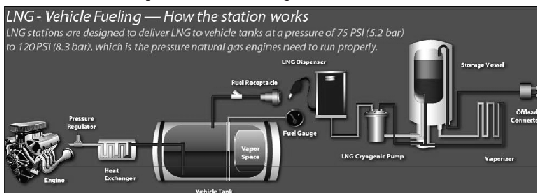
Figure 4: LNG Refueling Station Schematic
